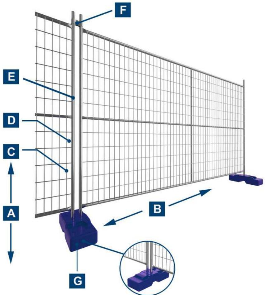
> hot dipped galvanized before welding or hot dipped galvanized after welding
